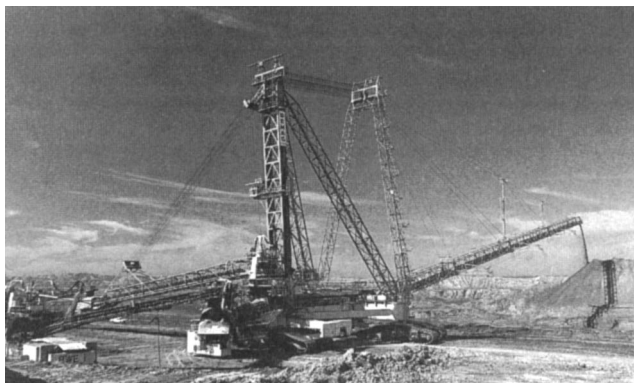
Fig. 14.3.6.5. Cross-pit spreader and BWE combination.
