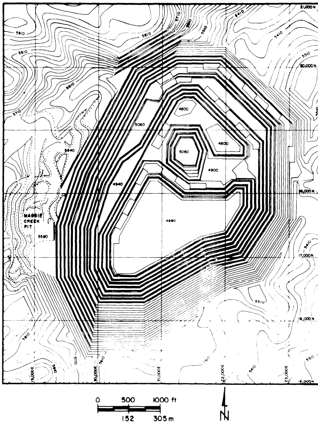
Fig. 14.1.2.3. Gold Quarry ultimate pit based on cone Z130 and $400 gold.
