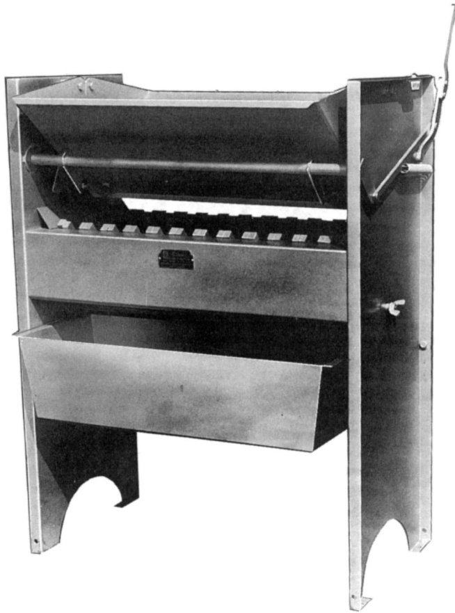
Fig. 5.3.5. Gilson adjustable sample splitter. (By permission of Gilson Screen Co.)
