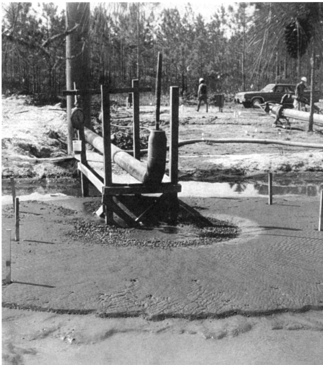
Fig. 22.4.9. Phosphate ore deposited at outlet of mining tool.
