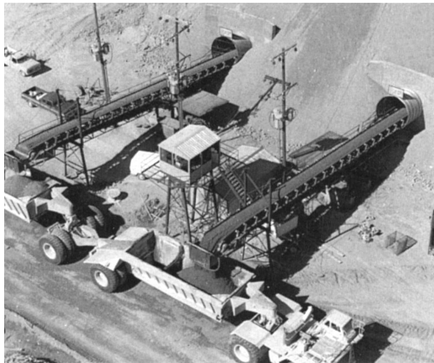
Fig. 25.2.21. Bottom-dump tandem trailers being loaded simultaneously by twin conveyor belts. Entire bottom is opened for discharge over receiving hopper (courtesy: Continental Conveyor Co.).
