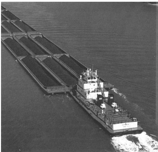
Fig. 25.2.34. Typical inland river 15-barge tow of 1500-ton (1360-t) capacity.
