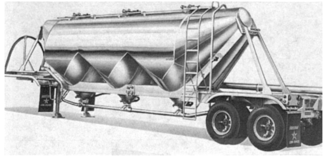
Fig. 25.2.22. Pressurized trailer with 1000-ft 3 (28-m 3 ) capacity allows air discharge of finely-sized mineral product via hose to overhead bins. Examples: cement, lime, etc. (courtesy: Fruehauf Co.).
