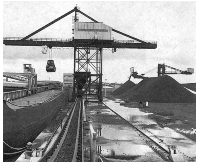
Fig. 25.2.29. Traveling clamshell grab bucket used to unload deep water vessels (courtesy: McNally-Wellman).
