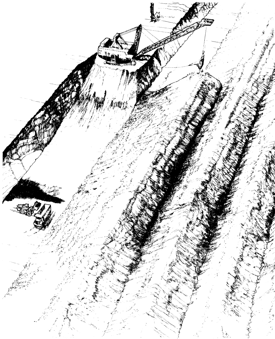
Fig. 14.3.0.1. Conventional area mining utilizing a dragline. (Anon., 1979; illustration by Frank Kulczak. By permission from Skelly and Loy, Harrisburg, PA.)
