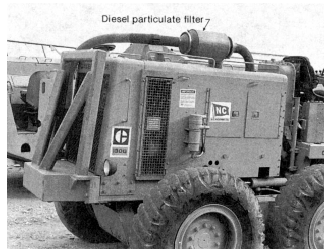
Fig. 11.5.6. Typical installation of a diesel particulate filter.
