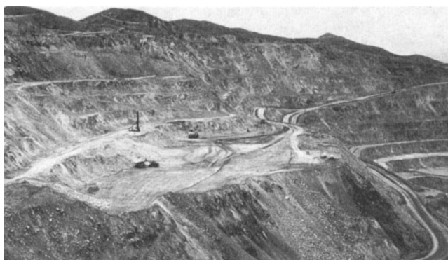
Fig. 14.1.4. Pushback in progress at a western US copper mine (1979).
