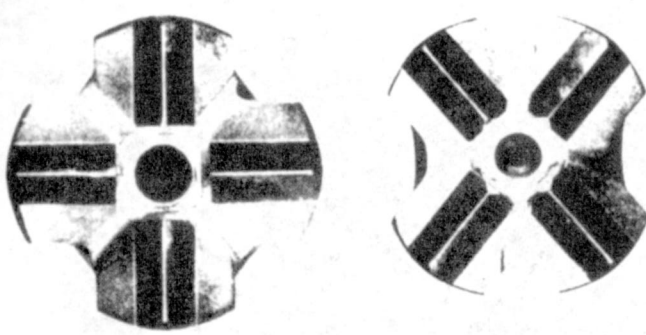
Fig. 9.1.28. Cross bit and X-bit (from Kurt, 1982, originally from Padley and Venables Ltd.).
