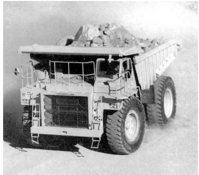
Fig. 9.3.5. Typical rear-dump mine haul truck (courtesy: Caterpillar Inc.).
