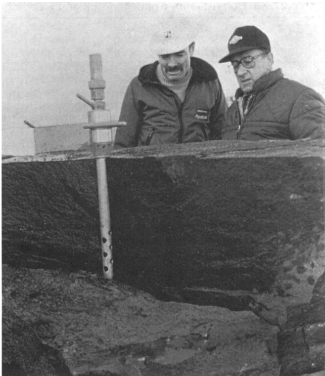
Fig. 22.9.19. Dresser basalt broken by pulse from 12-gage cartridge.
