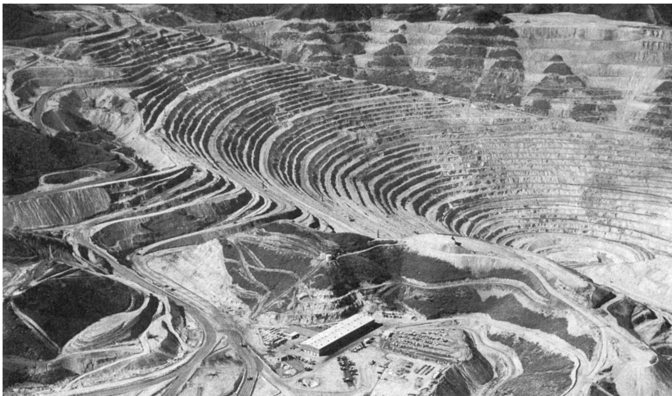
Fig. 14.1.2. Haulage ramp pattern in waste zone of a western US copper mine (1970).
