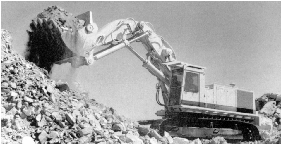
Fig. 9.3.1. Hydraulic excavator front shovel (courtesy: Caterpillar Inc.).
