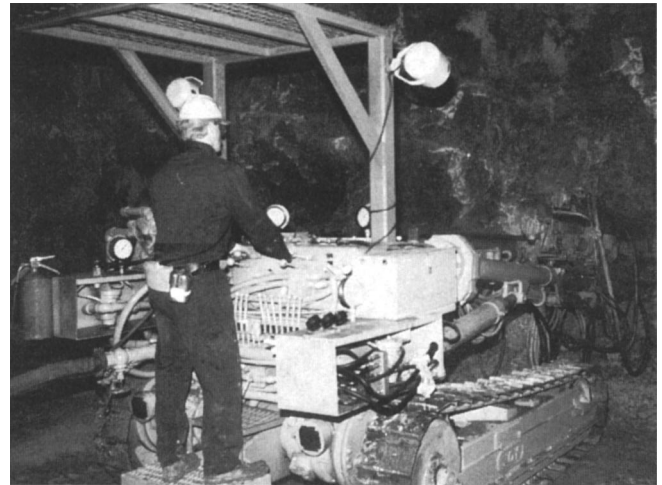
Fig. 22.9.6. Drill-split fragmentation apparatus.
