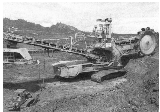
Fig. 13.3.16. BWE modern compact machine working in difficult overburden (courtesy: O&K Orenstein & Koppel, A.G., West Germany).
