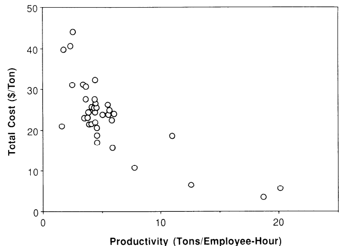
Fig. 23.3.4. Plot of cost survey results showing total cost vs. productivity for surface mining operations. Conversion factor: 1 ton = 0.9072 t.
