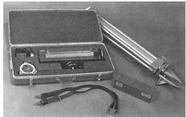
Fig. 10.3.53. Distance measuring system using two laser beams (courtesy: Aftgen).
