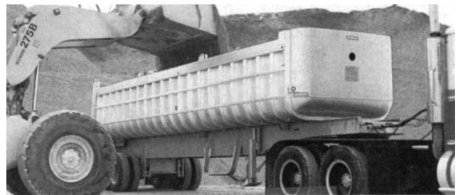
Fig. 25.2.19. Loading minerals into the frame-type trailer is done by front-end loader. Smooth interior avoids mineral buildup (courtesy: Fruehauf Corp.).
