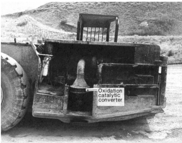
Fig. 11.5.4. Typical installation of an oxidation catalytic converter.
