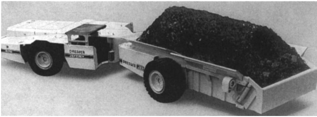
Fig. 17.2.16. Diesel-powered mobile handler. (Courtesy: Dresser Industries, Inc.)
