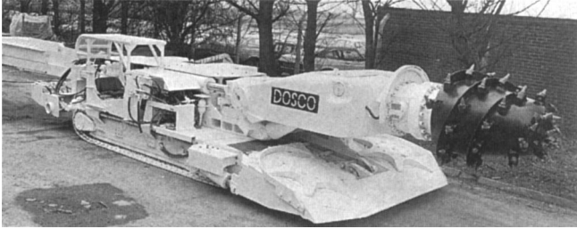
Fig. 17.2.15. Typical roadheader for use in coal or soft rock. (Courtesy: Dosco Corp.)
