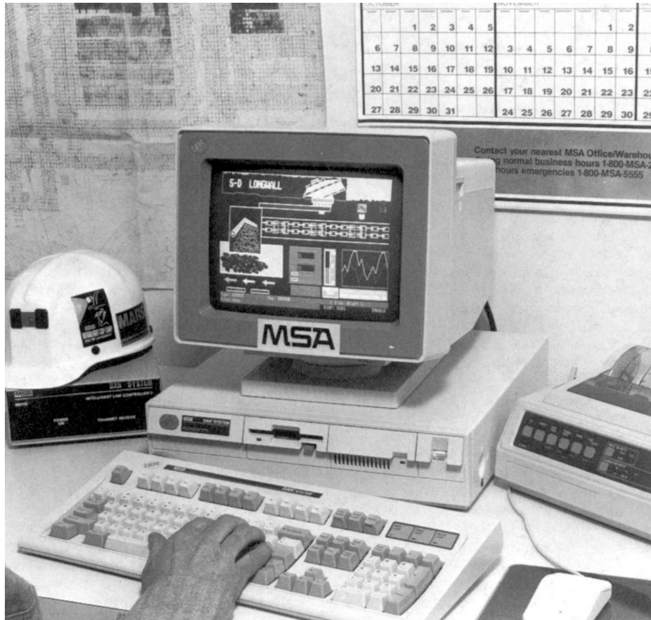
Fig. 12.6.4. A typical workstation for a mine monitoring system. (courtesy: Mine Safety Appliances Company).
