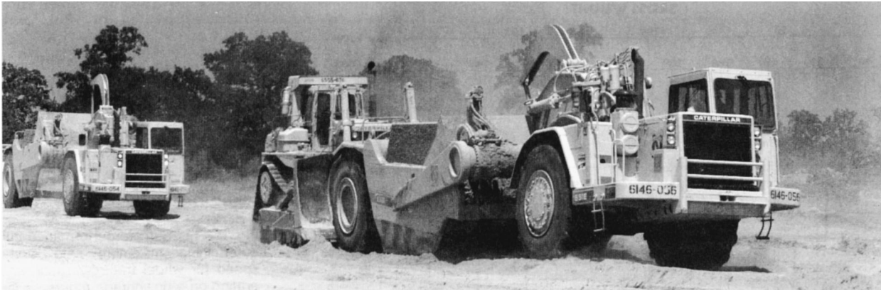
Fig. 9.3.12. Typical wheel tractor scraper (courtesy: Caterpillar, Inc.).
