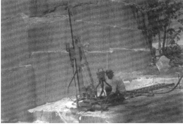
Fig. 14.2.1.3. Line drilling in the Friendsville quarry.
