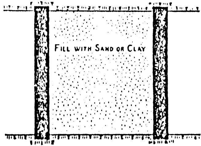
Fig. 11.6.3. Well-constructed explosion-proof stopping.
