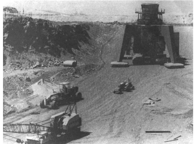
Fig. 13.5.7. Movable crusher in transit on crawler transporter (courtesy: Krupp International, Houston, TX).
