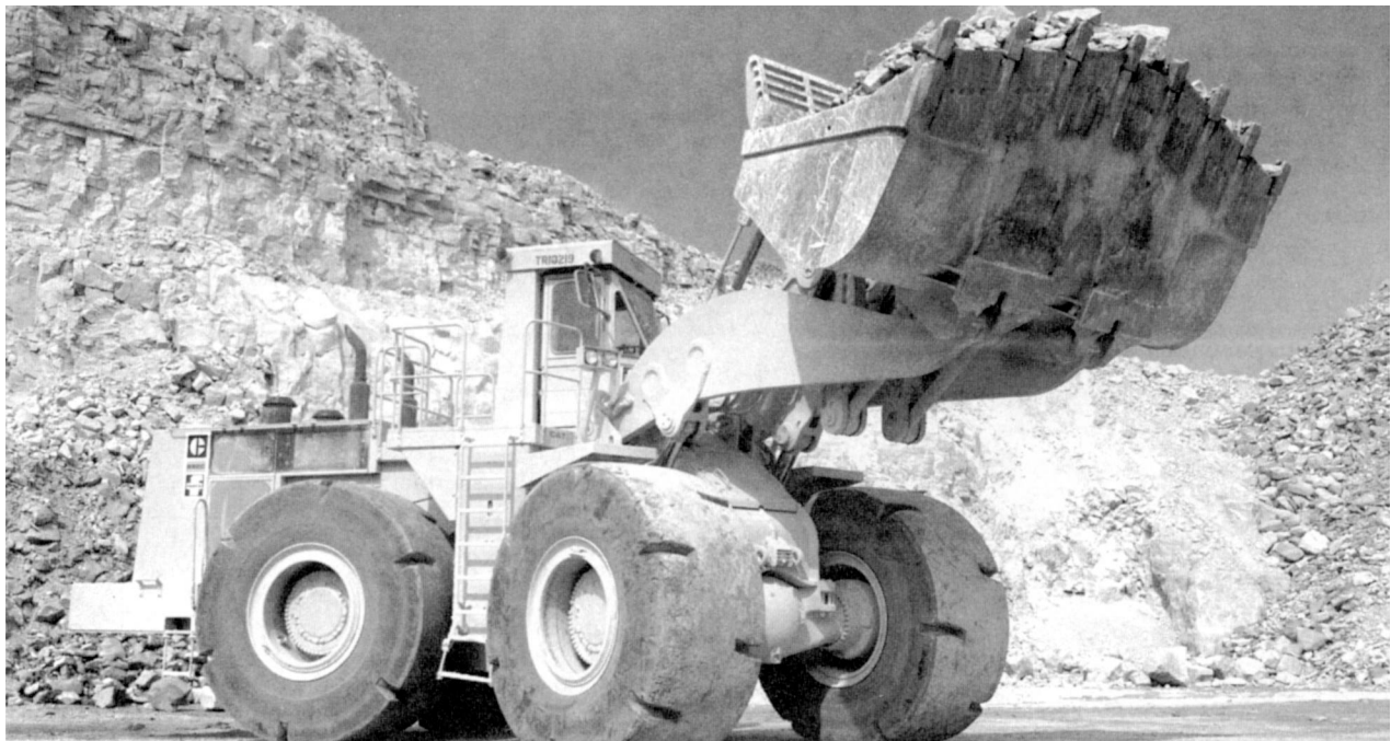
Fig. 9.3.3. Front-end wheel loader (courtesy: Caterpillar, Inc.).
