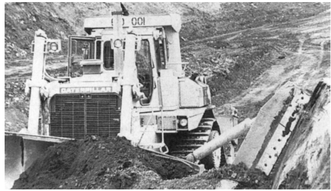
Fig. 14.1.5.5. Slope board used to recover thin, steeply dipping layers of ore.
