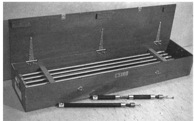
Fig. 10.3.29. Mini-frac equipment (courtesy: CSIRO).
