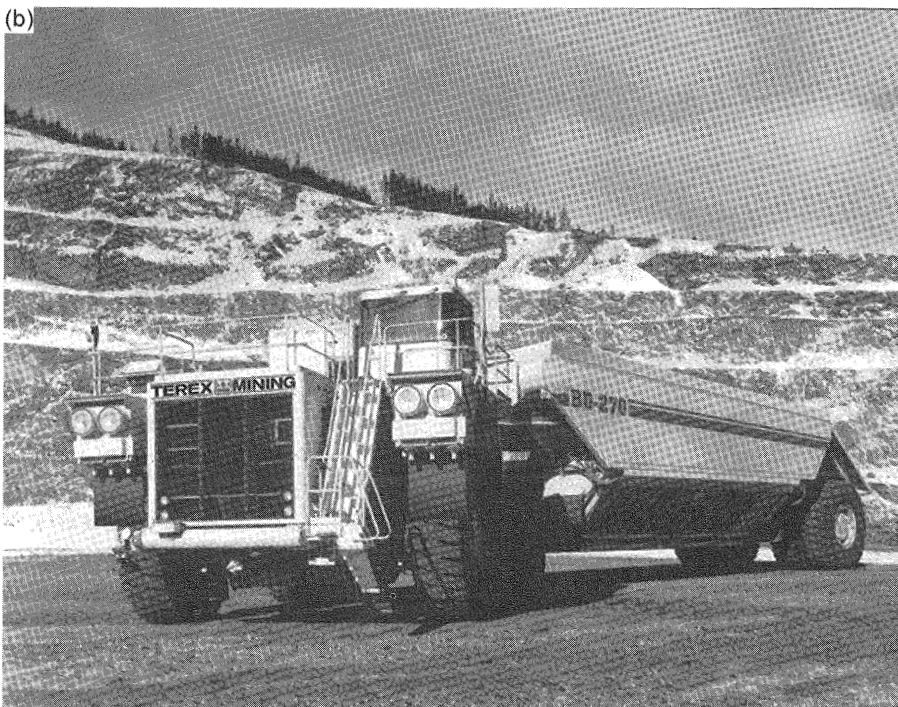
FIGURE 6.6. Unit operations and equipment for surface mining: rubber-tired haulage. (a) Diesel-electric rear-dump truck. (By permission from Terex Corporation, Westport, CT.) (b) Bottom-dump tractor-trailer. (By permission from Terex Corporation, Westport, CT.) (c) Wheeled scraper. (By permission from Terex Corporation, Westport, CT.) (d) Side-dump car. (By permission from Difco, Inc., Findlay, OH.) (e) Overland belt conveyor. (Photo courtesy of Continental Conveyor & Equipment Company, Winfield, AL.)
