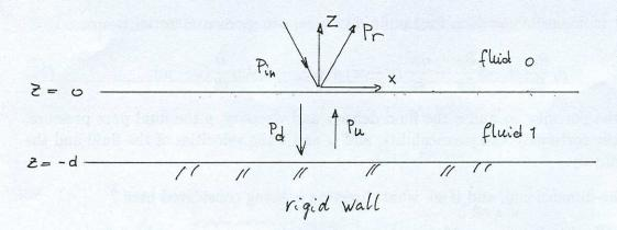
3) A plane monochromatic wave  $p_{in}$  impinges obliquely from above upon the interface between fluids 0 and 1 (see figure). The wave partially reflects  $(p_r)$  and partially transmits as a downgoing wave  $p_d$ . Fluid 1 is bounded from below by a rigid wall. Because of the reflection from the rigid wall, there must also be an upgoing wave  $p_u$ . Omitting the common factor  $\exp i(\omega t - k_x x)$  in all terms, the pressure in fluid 0 is written as:
