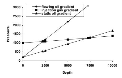
d) The valve setting pressures are 100 psi above the flowing well gradient
