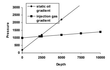
c) If the flowing well gradient is 0.15 psi/ft, then get , deepest injection point is given by d, where 200+0.15 d = 1000+0.04 d . So d = 800/0.11=7273 ft . Pressure = 100+0.4\*800/0.11=3009 psi
