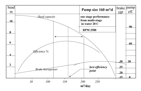
Use this curve and the Duns/Ros gradient curves to calculate the number of stages required for the pump.
