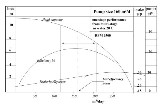
Use this curve and the Duns/Ros gradient curves to calculate the number of stages required for the pump. (1 psi = 6.89 kPa).
