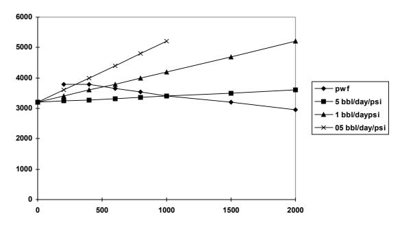
This the oil flow rate decreases steadily with time. According to the Duns/Ros curves, we expect it to stop completely when the II is about 0.5 bbl/day/psi, since then the flow is predicted to be unstable (slopes of equal sign). This prediction is not very certain, however.
