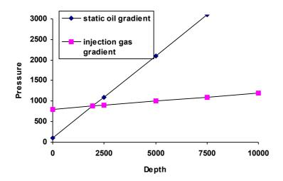
c) From the Duns/Ros gradient curve (3<sup>1</sup>/<sub>2</sub>" tubing, GOR 1000, watercut 0%) for production rate 1000 bbl/day, get the following pressures, assuming 250 psi tubing head pressure
