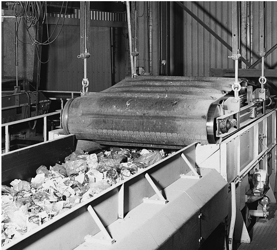
Fig. MS.1 - Magnetic separation of ferrous metal from mixed MSW
