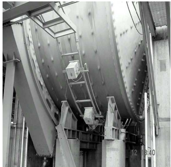
Fig. 3.3.15d - SAG mill ball trajectories landing on the load and striking the mill liners (l); Microphones of the Imactmeter on the shell of the SAG mill [Almond, 2005].
