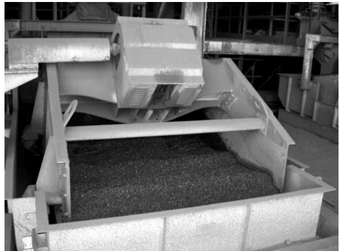
Fig. 1.8.10 - Flip Flow screen (l). Dewatering screen for mid-size coal (r) [Schubert Vol. 1 / TU Delft].
