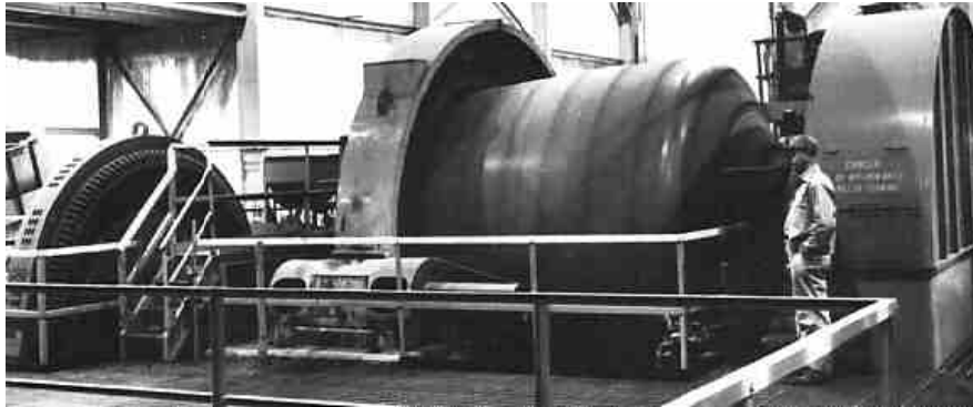
Fig. 3.3.6 - Ball mill with gear/pinion assembly (middle) and driving motor (left) [SME].
