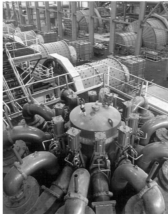
Fig. 2.6.3 - Bank of cyclones for small cut sizes (l), or high capacity in a grinding circuit (r) [Amberger Kaolinwerke / Krebs Engineers].
