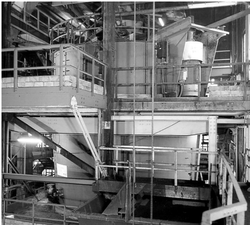
Fig. 2.4.3 – Centrifugal classifier (“deduster”) for raw small coal can handle dry as well as moist feed
