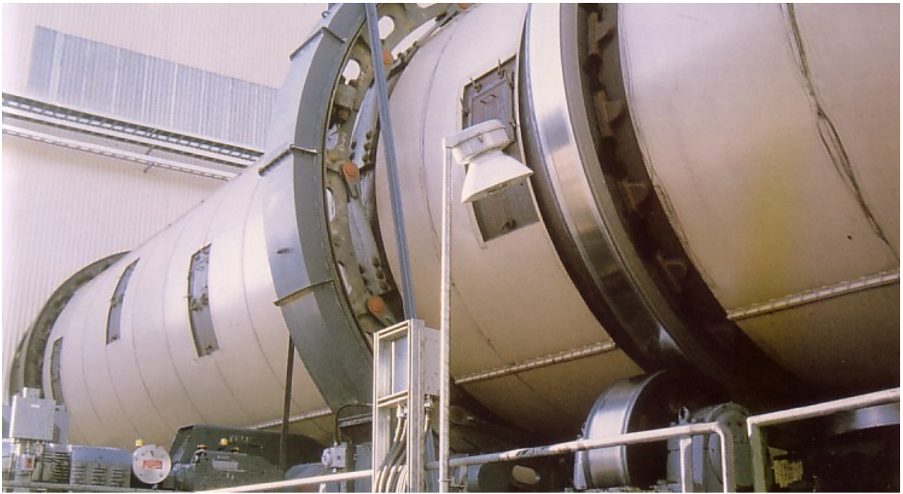
Figure 10 - Coal rotary dryer [KHD Humbold Wedag]
