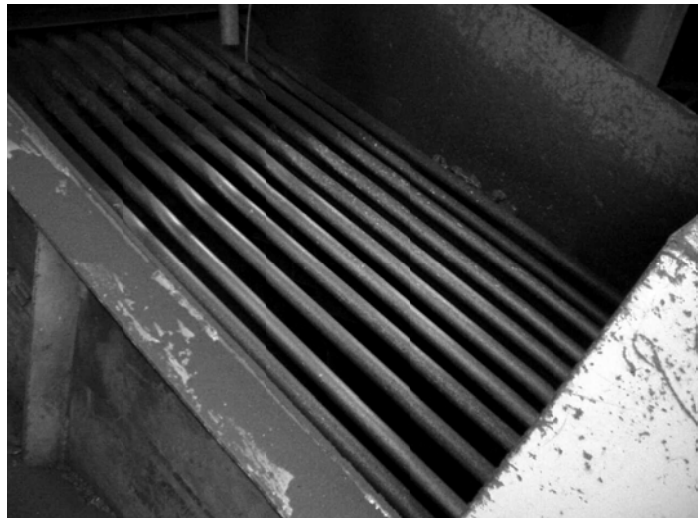
Fig. 1.8.2 - Ore grizzly, schematic (l). 50 mm static grizzly installed directly preceding a jaw crusher at the coal preparation plant of Dr. A. Schäfer Bergbau GmbH, Germany (r) [Wills / TU Delft].
