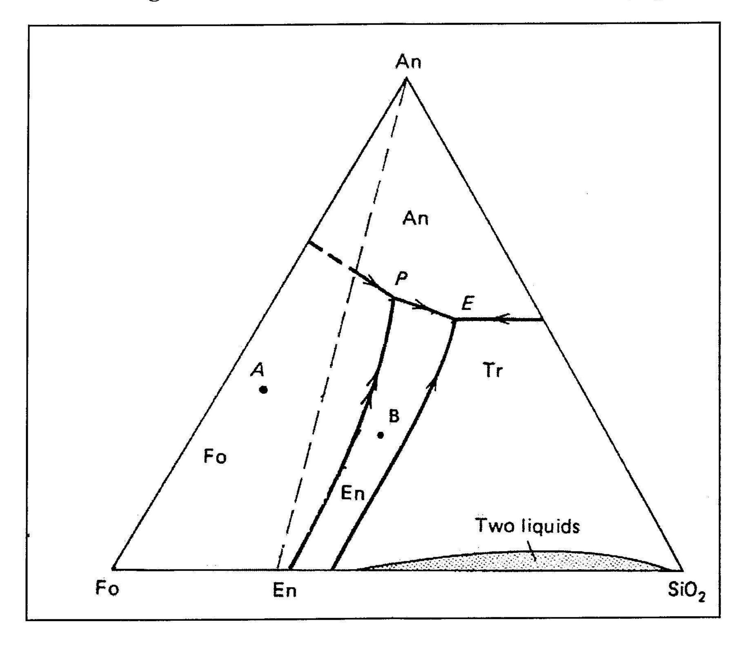
The diagram shows the liquidus projection of the system forsterite-anorthite-silica  $(Mg_2SiO_4-CaAl_2Si_2O_8-SiO_2)$  at a certain temperature. The phases in this system are:
