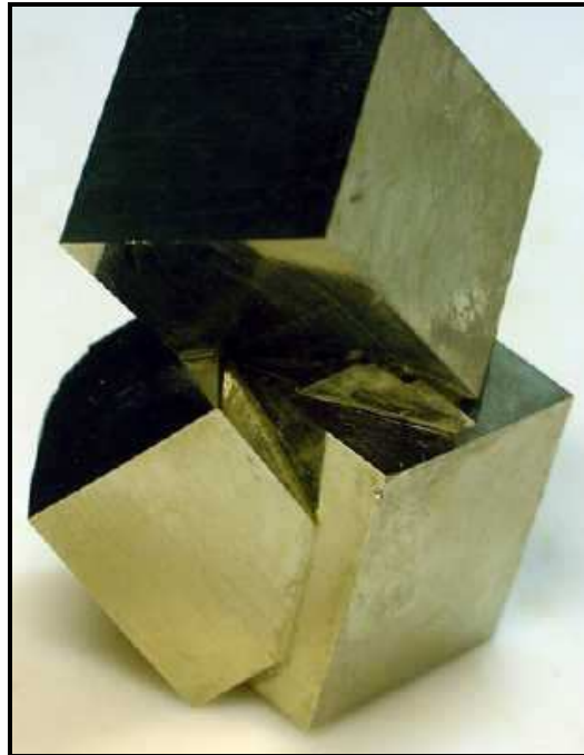
Isometric crystals of pyrite.
