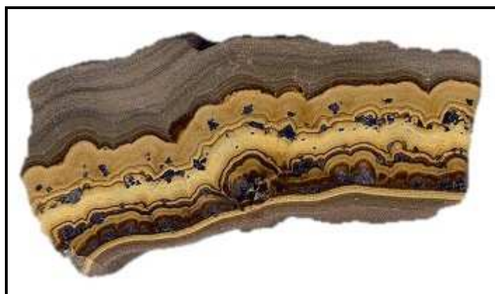
Colloform texture in a polished hand specimen.
