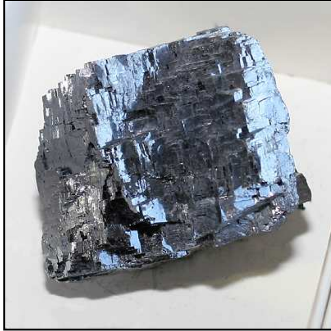
Galena. Three perpendicular cleavage directions are clearly visible.
