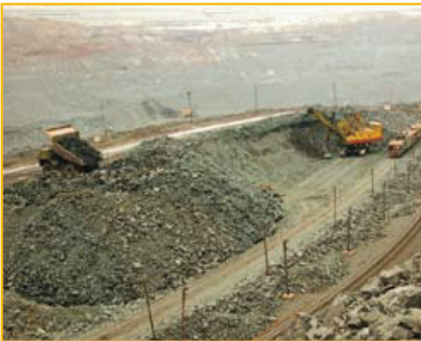
Rehandling of ore – a temporary stockpile is made.
