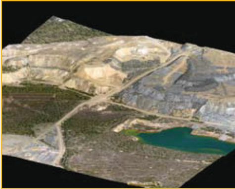
Image created in Surpac showing historic workings at Hannukainen, Finland using laser scanned DTM and orthophotos.
