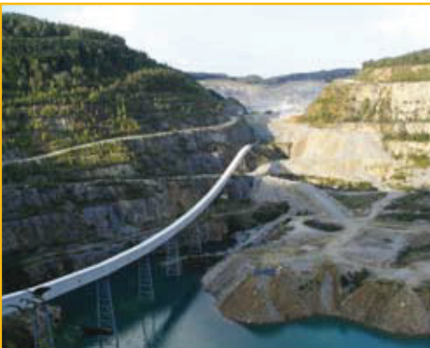
Conveyor belt between the Rohdenhaus crusher and washing plant.
