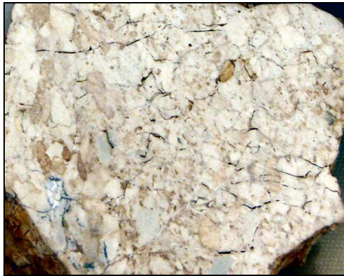
Fig. 3.51. Mullite, white, formed after kaolinite as a result of baking by an underground coal fire, Mnt Wingen, Australia
