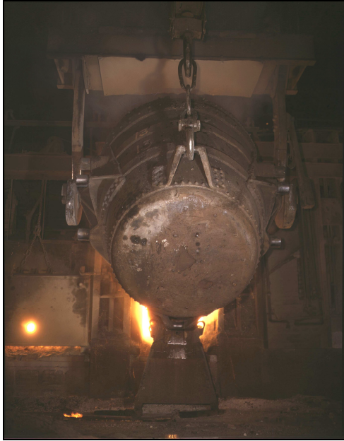
Figure 3.31. A ladle charging a steel converter. The refractory lining of the ladle is partly made of magnesia-containing bricks
