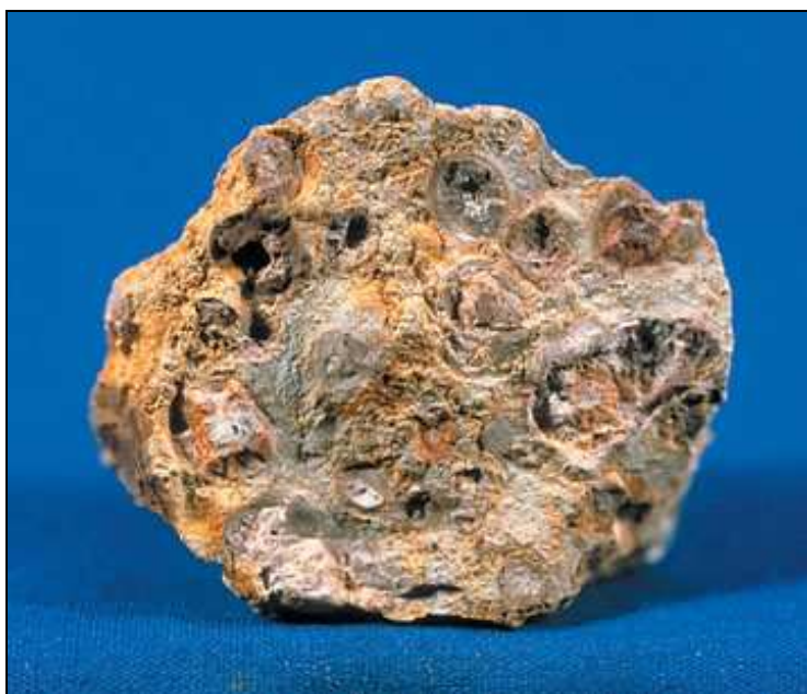
Fig. 2.38. Bauxite. Reddish colours indicate iron hydroxides such as goethite. Very pure bauxite is white. The iron content of bauxite is one of its critical parameters.
