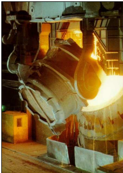
Figure 3.37. A ladle charging a steel converter. The ladle lining is partly made of pyrophyllite-containing bricks
