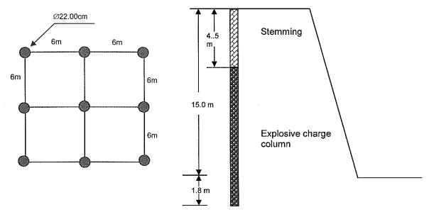
A traditional rotary drilling system is used at this mine for rock breakage with the blast pattern being B  $\times$  S = 6m  $\times$  6m pattern and each hole has a 1.8-meter sub-grade drilling (refer to the sketch). Site drilling tests suggest that
