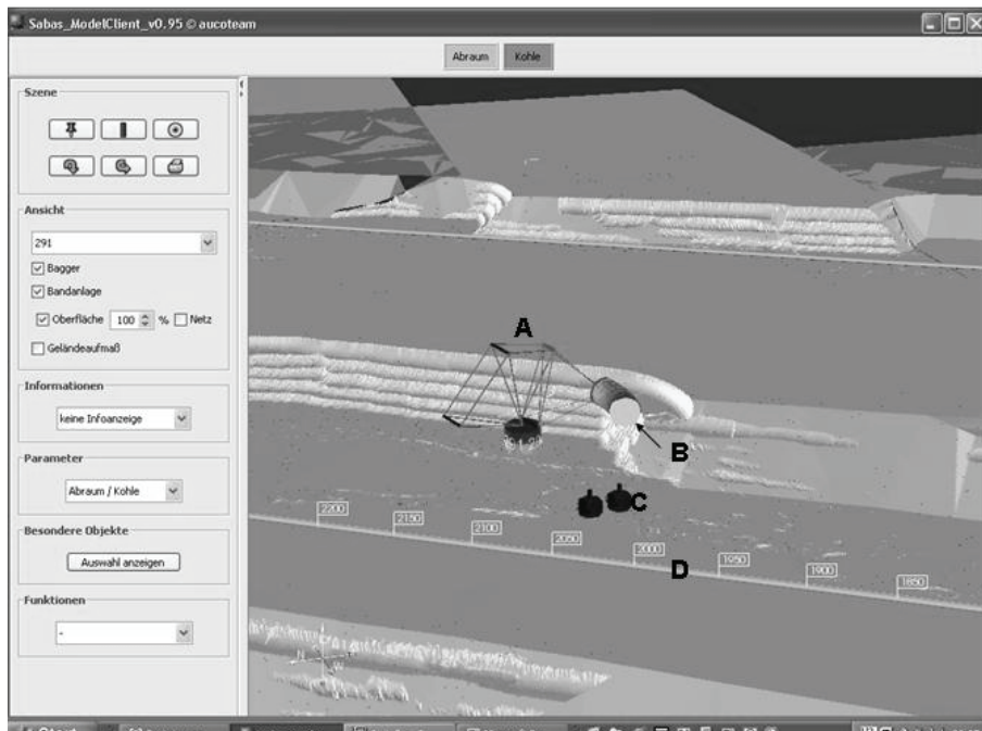
Figure 5 Screenshot of the desk visualisation of the digital mine showing the BWE (A), the position of the BWE along the conveyor belt (D), the slice the BWE is excavating (B) and the position of two pieces of auxiliary equipment (C). In addition to this information the position of wells, the geology from the geological model, the mine plan etc. can be visualised.
