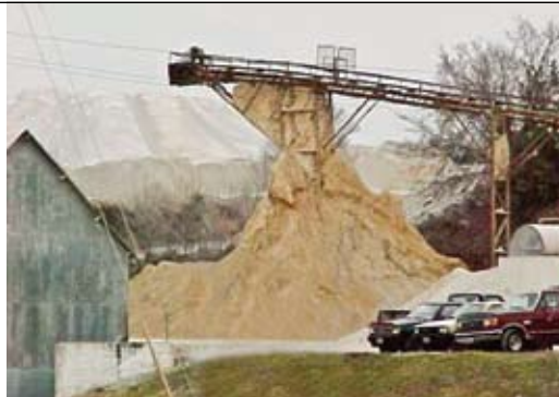
Figure 14.9 Even a modest amount of carryback left on the belt can accumulate to significant piles under the conveyor.
