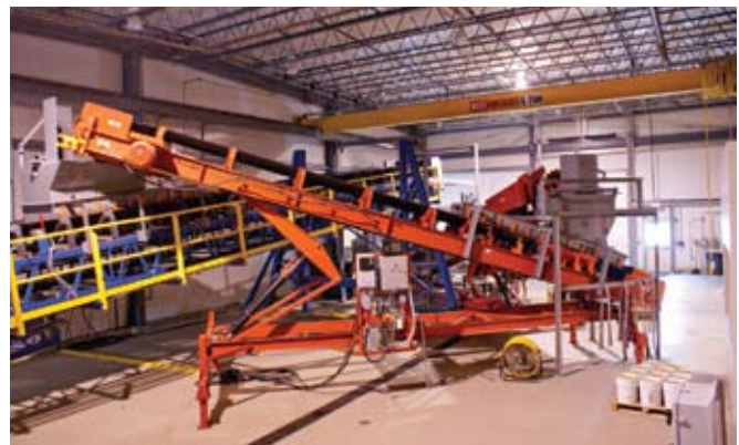
A three-part recirculating conveyor system at Martin Engineering's Center for Bulk Materials Handling Innovation allows for full-scale materials handling testing.
