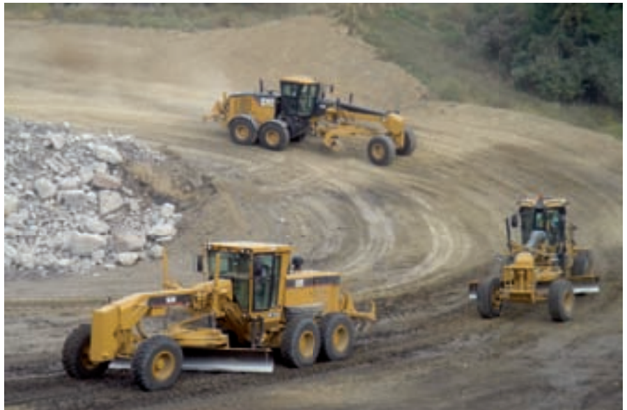
Two generations of Caterpillar graders at its Illinois test area – the 163H and the latest 14M joystick-controlled machine
