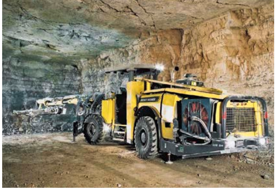
Rocket Boomer L1 C-DH drilling the face at Auersmacher limestone mine.
