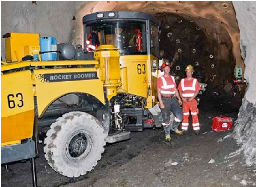
Atlas Copco equipment, such as this Rocket Boomer M2 C drill rig, plays a central role, pictured here with instructor Lars-Olov Jansson (left) and operator Noel Dunphy.
