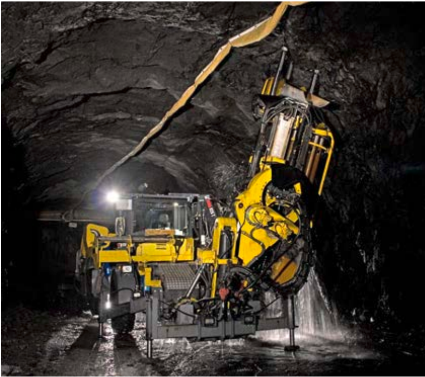
Simba W6 C drilling upholes at Kiruna mine.
