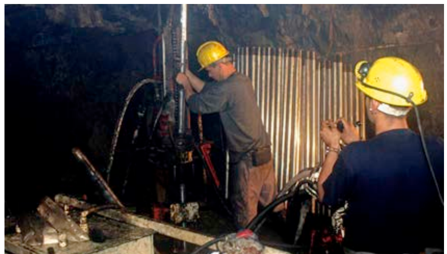
Core drilling in the levels.
