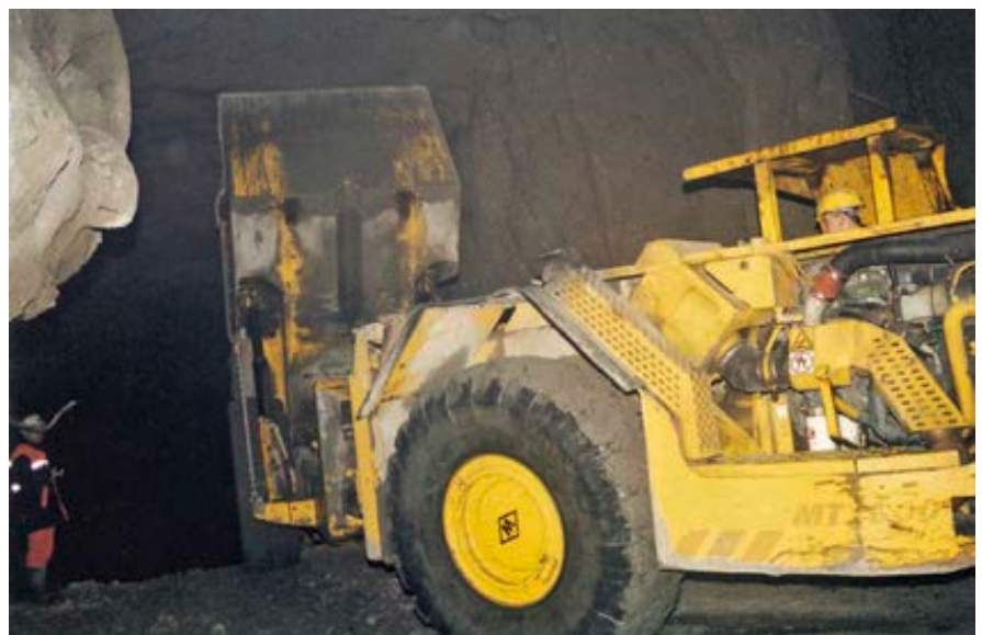
Minetruck MT2000 discharges cemented backfill into a primary stope.
