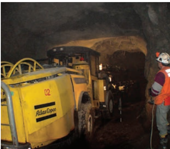
Rocket Boomer M2 C underground.
