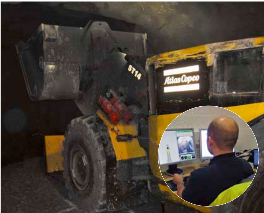
The Scooptram ST14 during tests at Kemi Mine, trams automatically between loading and dumping. The process is supervised from a remote control station.
