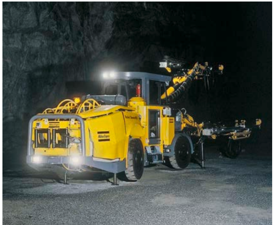
Rocket Boomer M2 C developing the sublevels.
