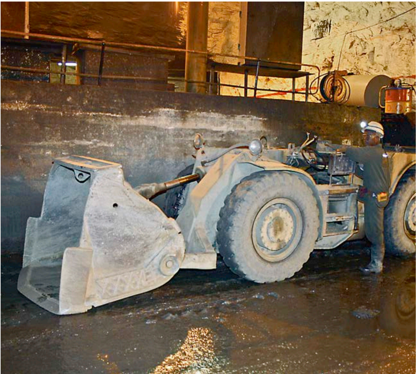
An Atlas Copco Scooptram ST2D, more than 20 years old, is still going strong with no apparent oil/hydraulic leaks or excessive emissions at the Otjihase mine.
