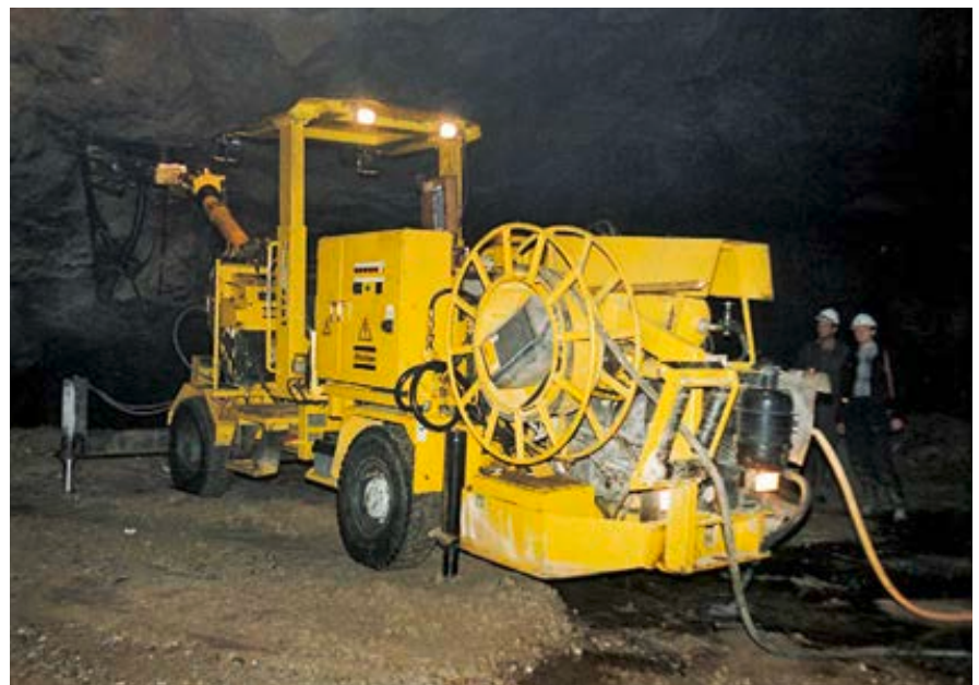
Rocket Boomer 281 drilling a crosscut entry.
