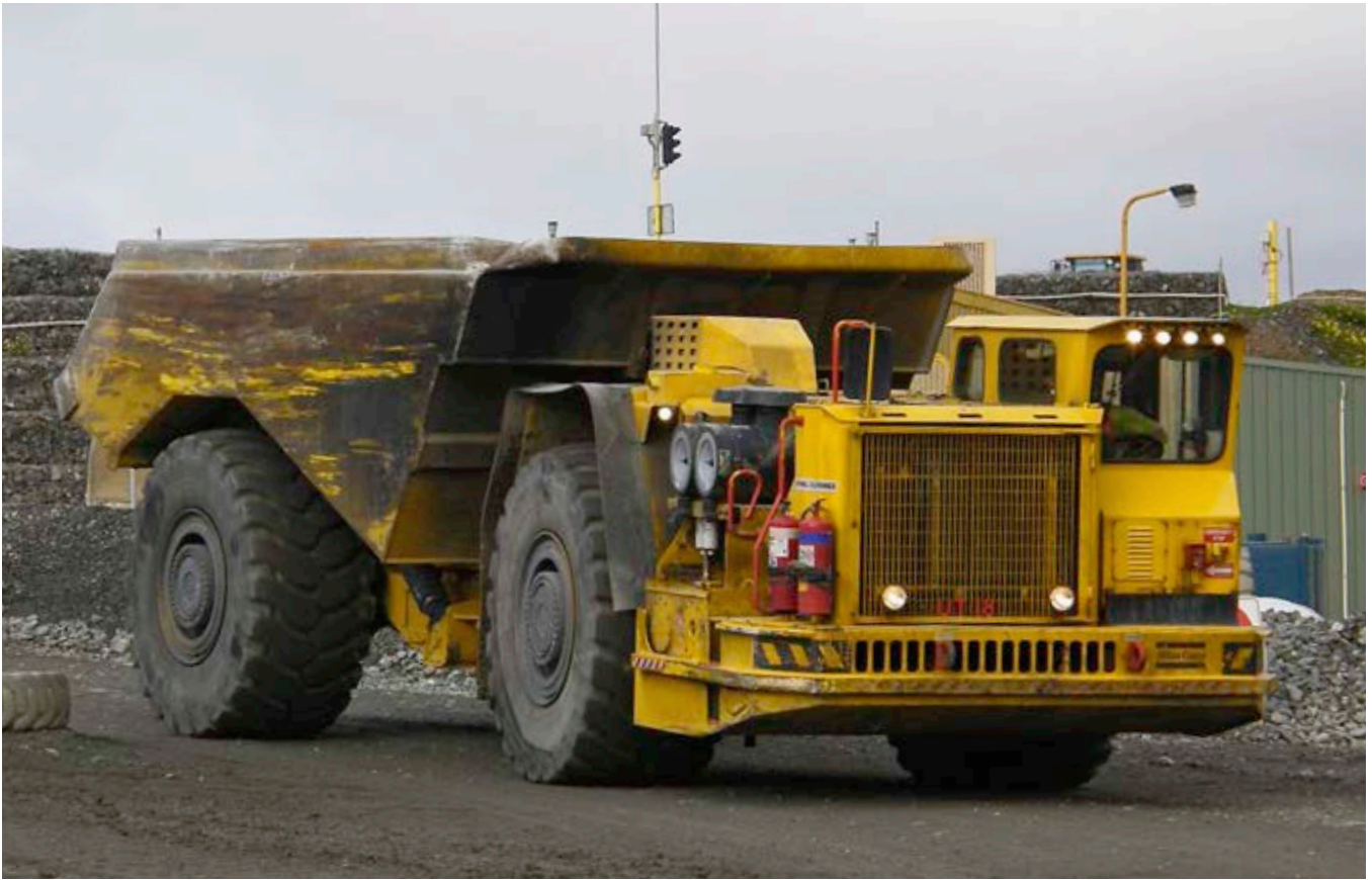
Minetruck MT6020 during the field test at Stawell Gold Mine in Australia.
