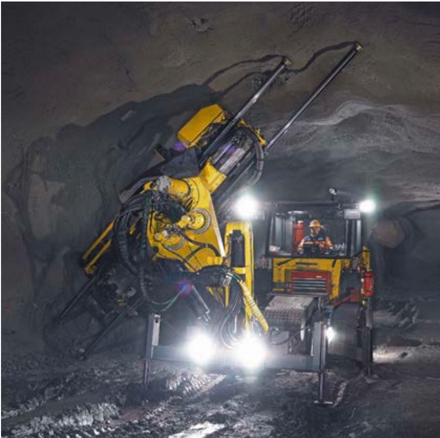
Simba M6 C at work in the sublevels at Kemi mine.
