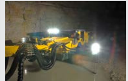
Rocket Boomer S1 L, the cabin version.
