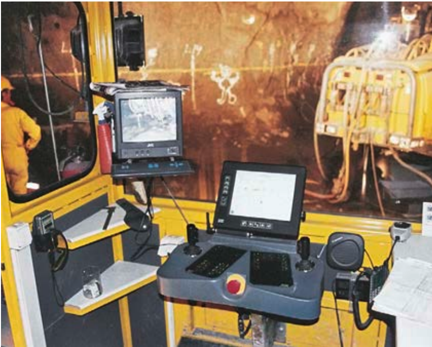
Ergonomically-designed cab on the Simba M4 C drill rig.
