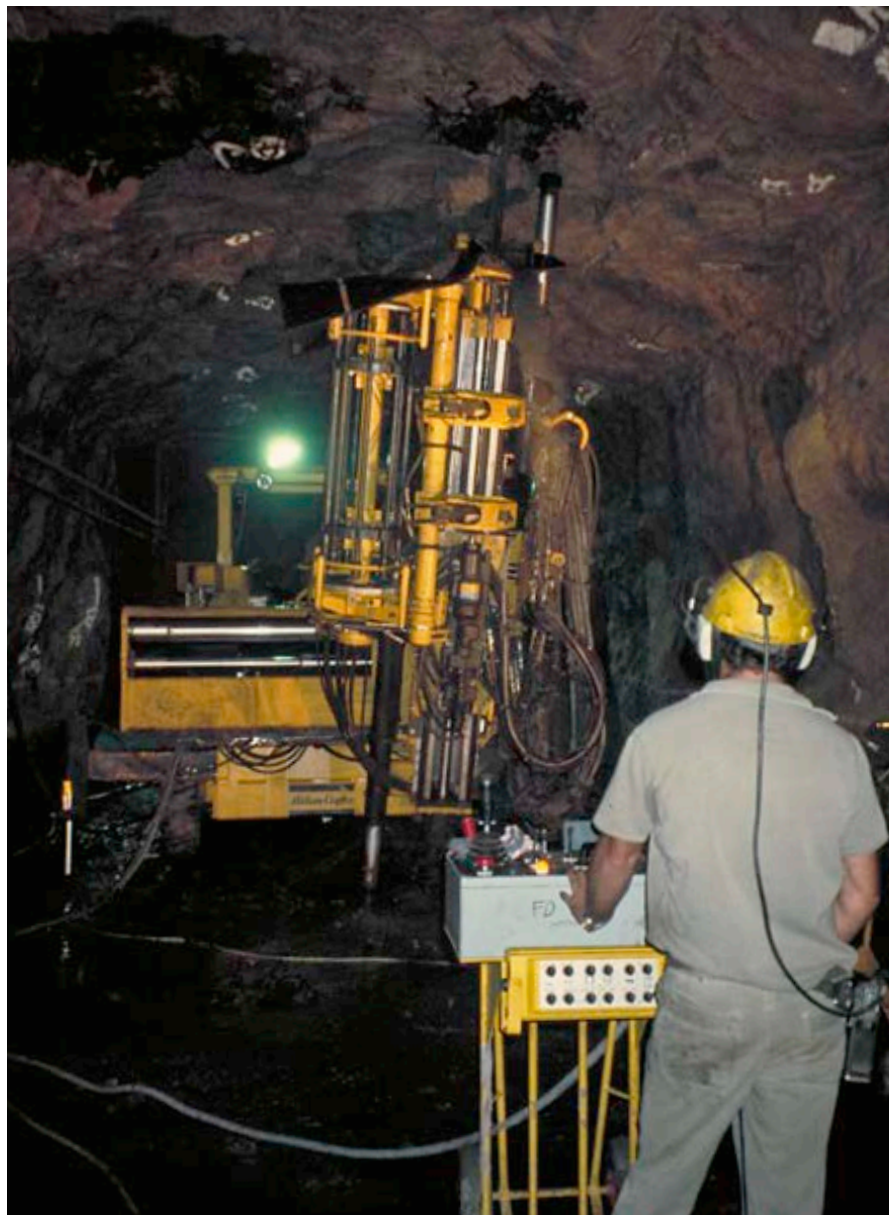
Simba H254 (the photo shows another rig than the one at Meishan).
