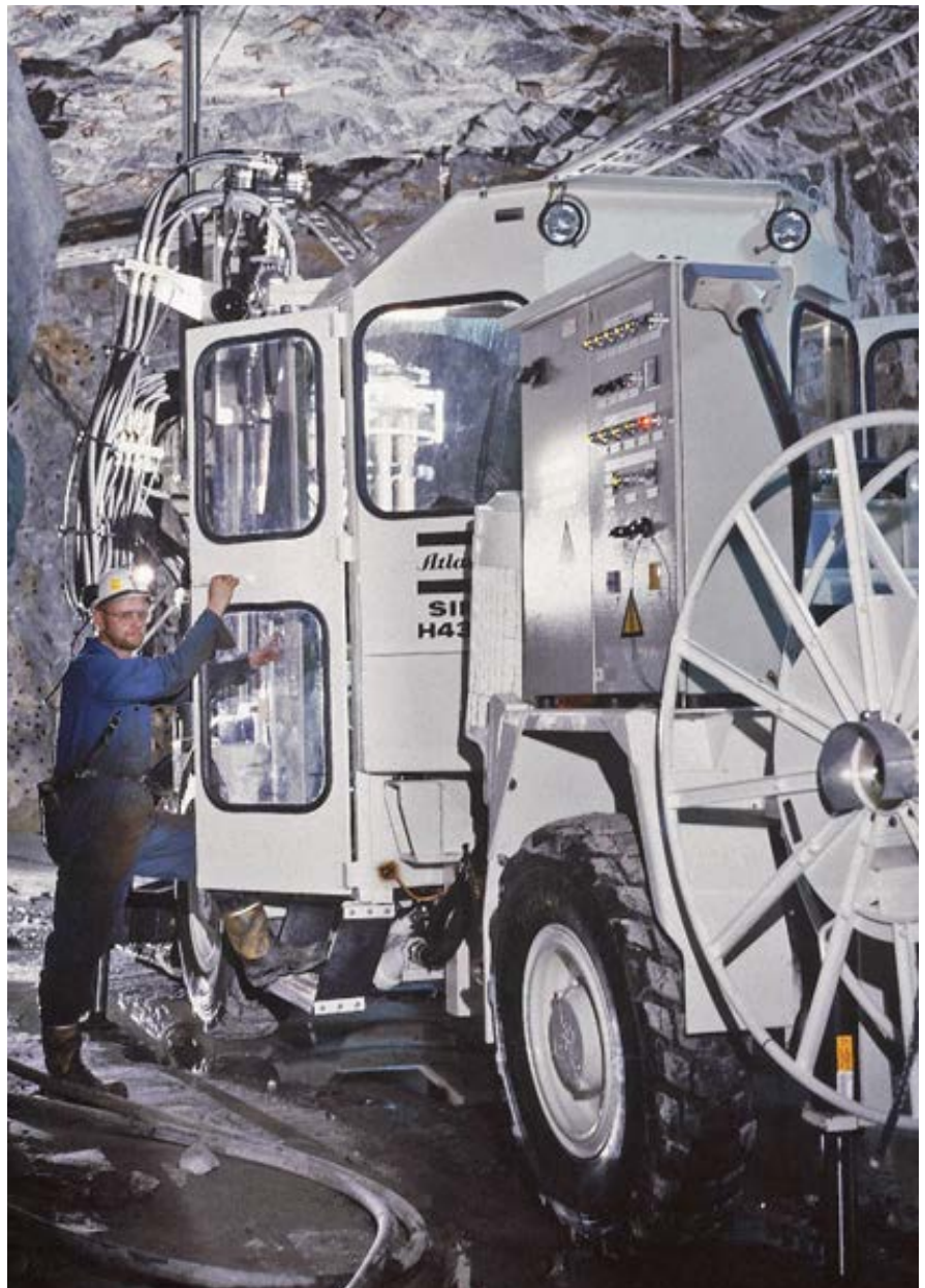
Simba 4356S longhole drill rig with COP 4050 tophammer rock drill.
