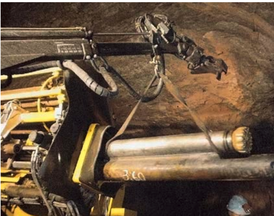
Simba MC 6-ITH with slot hammer.
