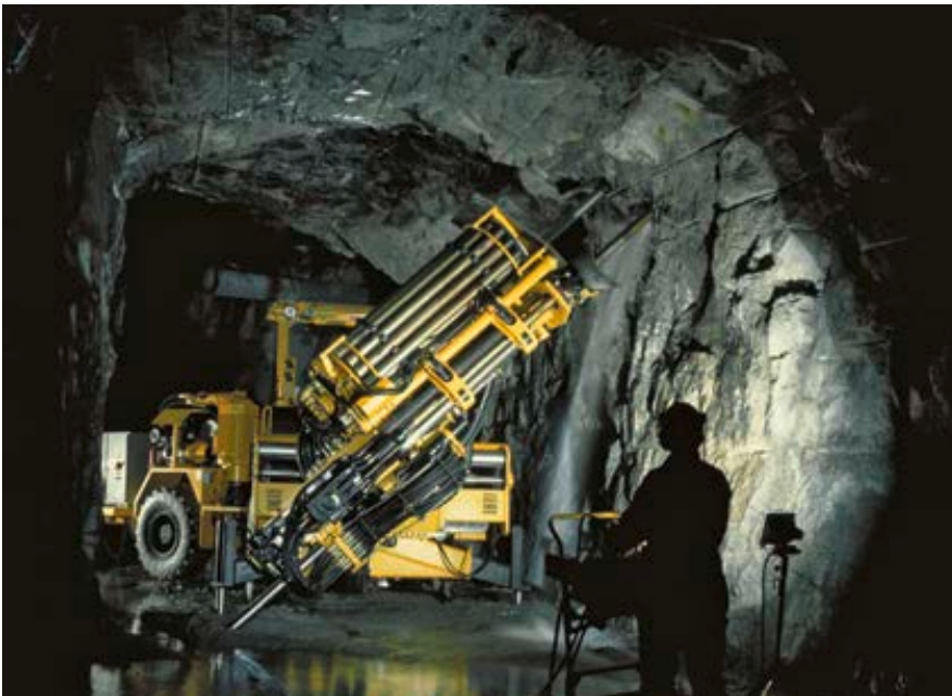
Simba H4353 long hole drill rig with COP 4050 rock drill.
