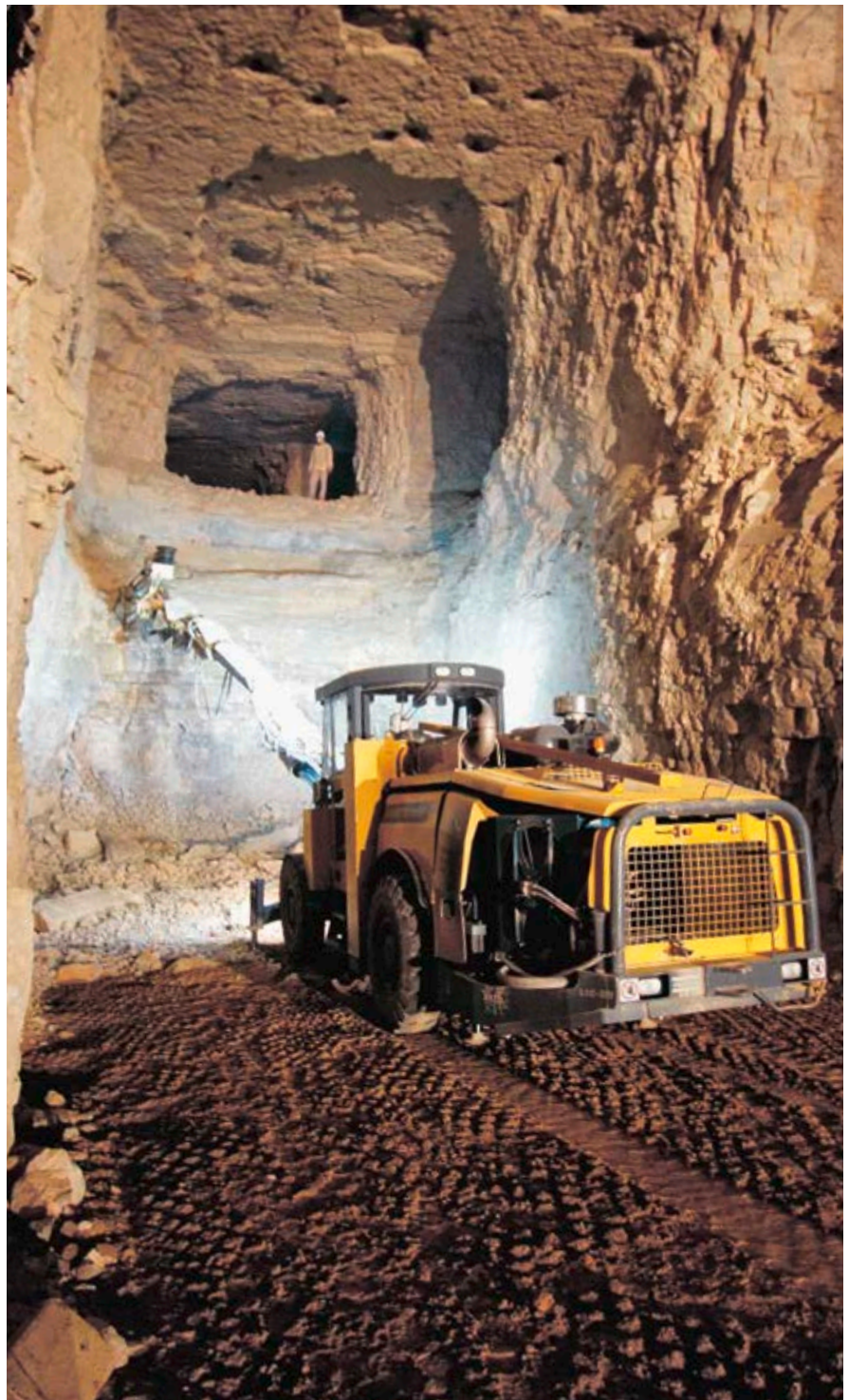
Rocket Boomer L1 C-DH with COP 1838HF rock drill achieves 8 m/min at Josefstollen.
