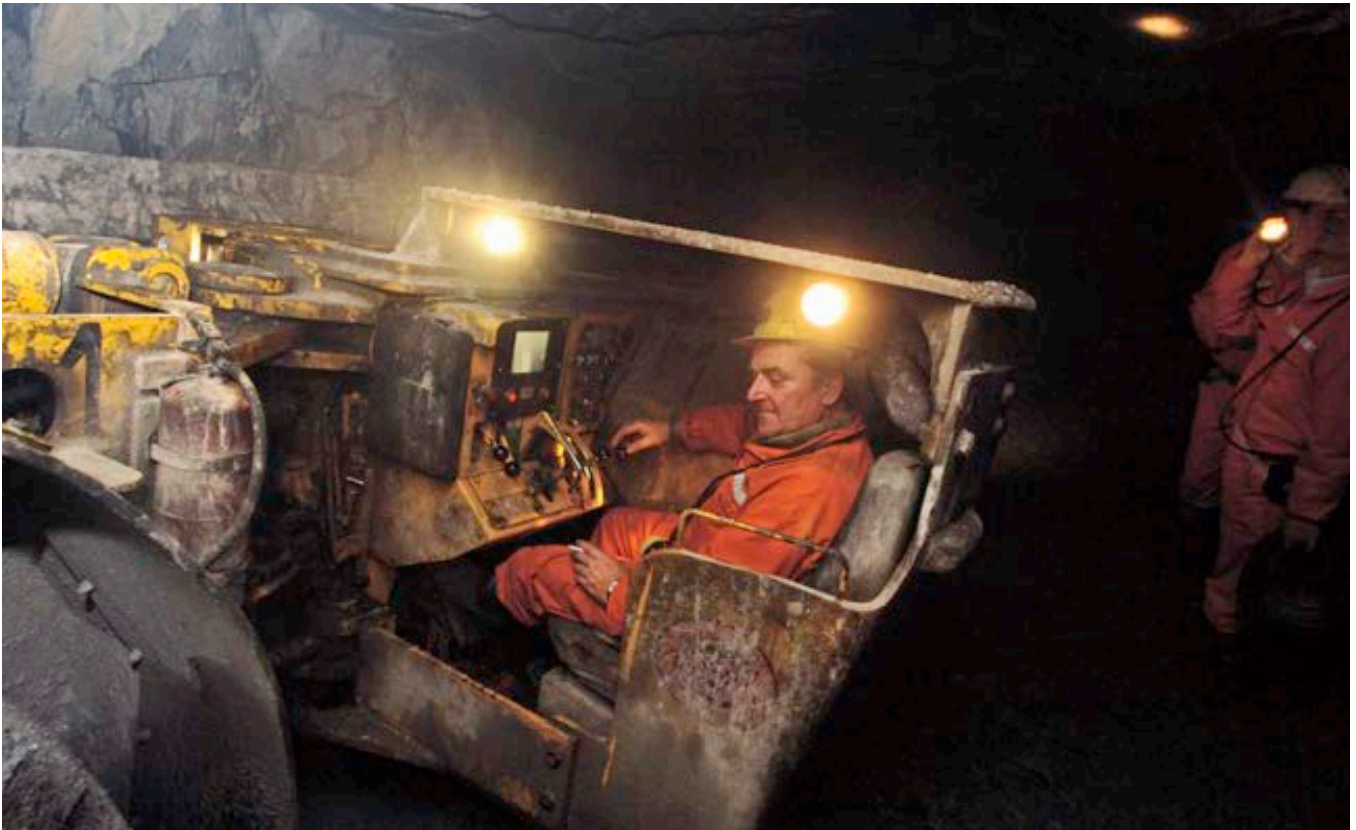
Scooptram ST600LP in low headroom stope.
