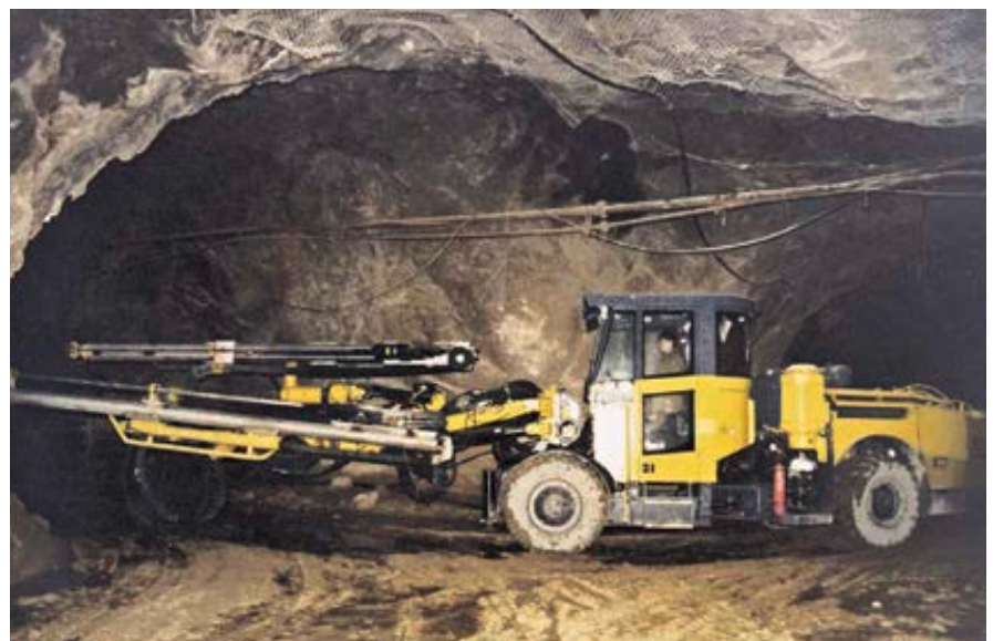
Rocket Boomer M2 C moving towards the faces.
