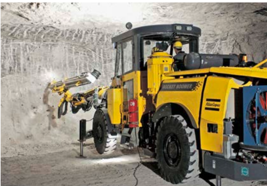
Rocket Boomer L1 C drilling 4.5 m-long blastholes at Obrigheim.
