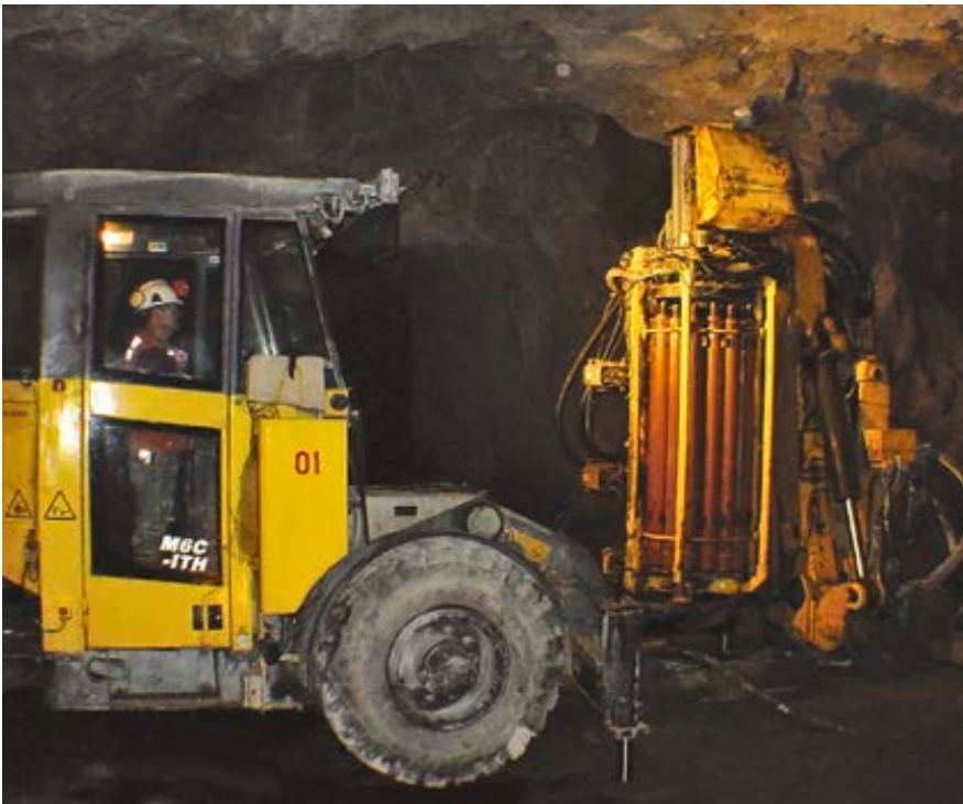
Simba M6 C drilling radial holes.
