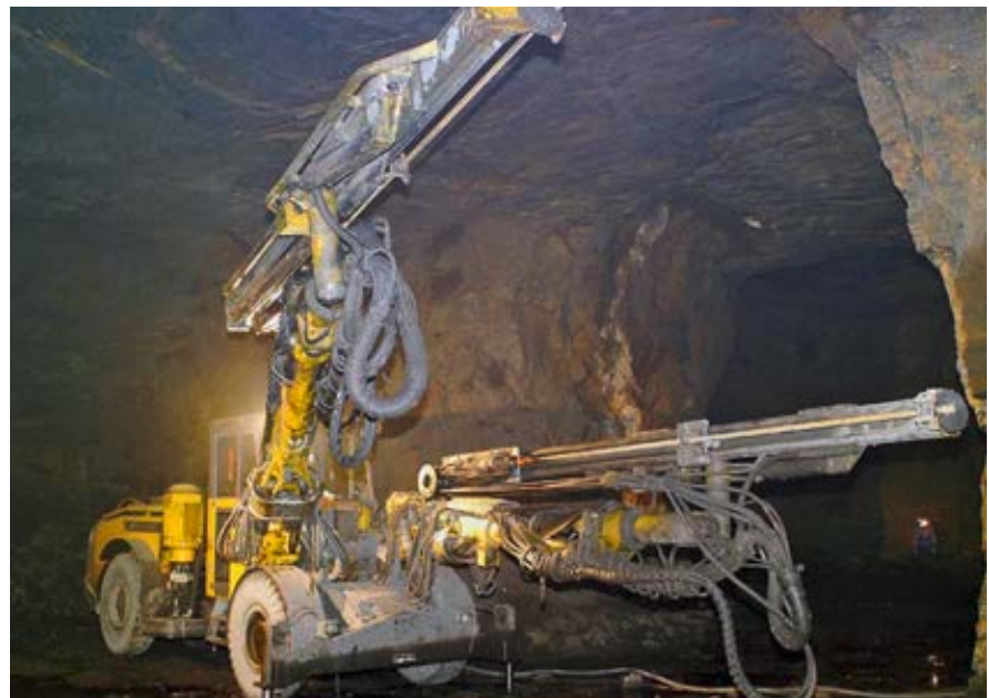
Rocket Boomer L2 C drill rig with COP 1838 rock drills at Madero mine.
