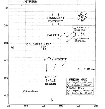
This crossplot may be used to help identify mineral mixtures from Sonic, Density, and Neutron logs. (The Neutron log used in the above chart is the CNL\*.) Except in gas-bearing formations, M and N are practically independent of porosity. They are defined as:
