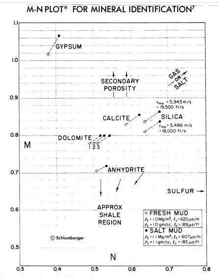
This crossplot may be used to help identify mineral mixtures from Sonic, Density, and Neutron logs. (The Neutron log used in the above chart is the CNL\*.) Except in gas-bearing formations, M and N are practically independent of porosity. They are defined as:
