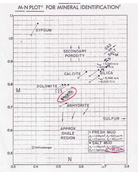
This crossplot may be used to help identify mineral mixtures from Sonic, Density, and Neutron logs. (The Neutron log used in the above chart is the CNL\*.) Except in gas-b\_aring formations, M and N are practically independent of porosity. They are defined as:
