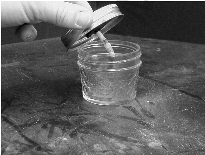
Figure 10.15 (a) Schematic drawing and (b) photograph of typical laboratory set up for measuring total soil suction using thermocouple psychrometer.
