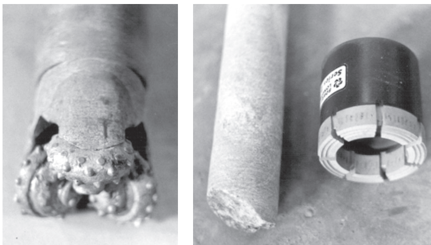
Figure 4.7 Three-cone roller bit (left). Rock coring bit and segment of rock core (right).
