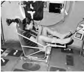
FIGURE 13.38 Astronaut Tamara Jernigan uses a body mass measuring device in the Spacelab Life Sciences Module (Passage Problems 85–88)
