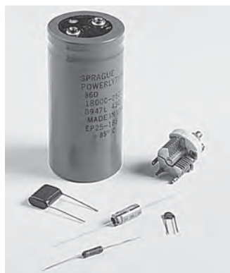
FIGURE 23.5 Typical capacitors. The large unit is an 18-mF electrolytic capacitor. At top right is an air-insulated variable capacitor in which one set of plates rotates to change the capacitance. The smaller capacitors range from 43 pF to 10 \mu F.
