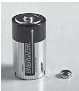
FIGURE 25.6 Both batteries are rated at 1.5 V, but they have different internal resistances. Which do you think has the higher R_{\text{int}} ?
