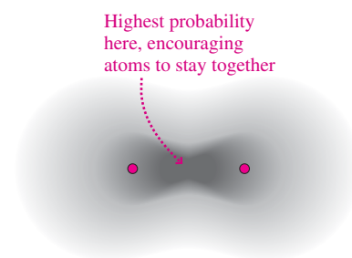
FIGURE 37.4 Probability density for finding electrons in the ground state of molecular hydrogen ( \text{H}_2 ).
