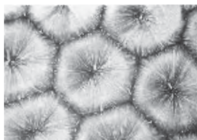
FIGURE 16.10 (a) Convection between two plates at different temperatures. (b) Top view of convection cells in a laboratory experiment. Fluid rises at the centers and sinks at the edges of the hexagonal cells.
