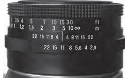
FIGURE 31.37 A 35-mm camera lens (Passage Problems 82–85). The numbers from 22 to 2.8 at the bottom are values for the f -ratio, f/d . Turning the ring with these numbers adjusts the iris that covers the outer part of the lens, thus changing the f -ratio.
