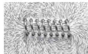
FIGURE 26.36 Iron filings trace the magnetic field of a loosely wound solenoid. Compare with the field of a bar magnet shown in Fig. 26.1.
