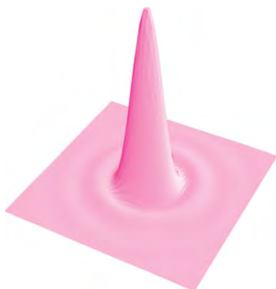
FIGURE 32.27 3-D plot of intensity versus position in circular diffraction. The right-most image in Fig. 32.26 shows the corresponding diffraction pattern.
