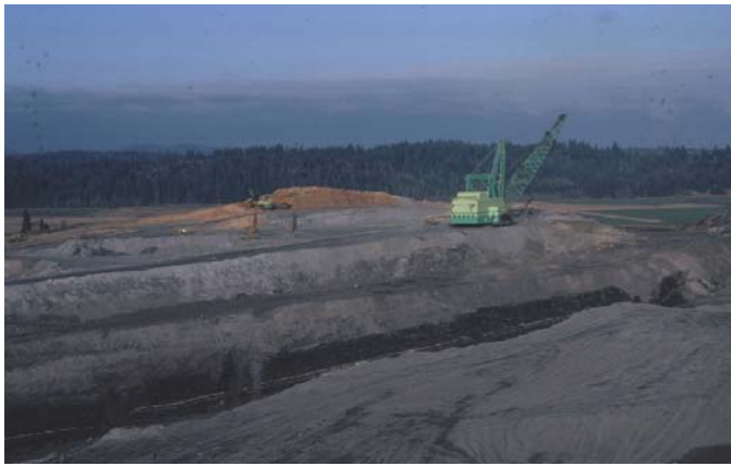
Figure 4.9 Dragline stripping coal operation
