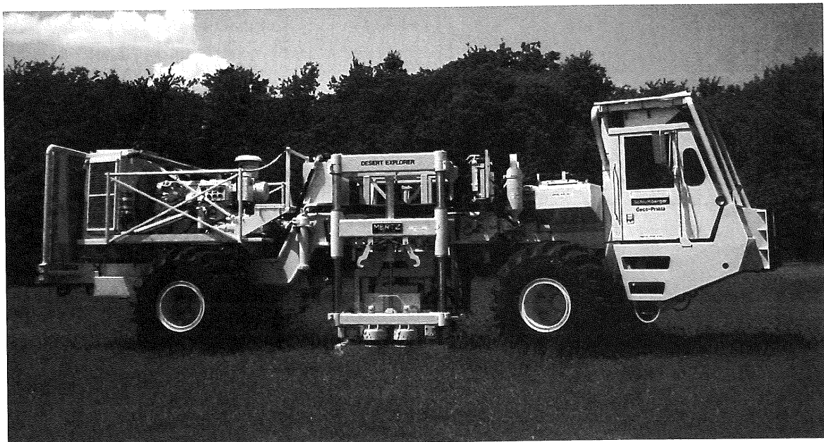
Figure 7.18 A truck for Vibroseis surveying.
