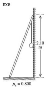
A 10.0-kg uniform ladder that is 2.50 m long is placed against a smooth vertical wall and reaches to a height of 2.10 m, as shown in the figure. The base of the ladder rests on a rough horizontal floor whose coefficient of static friction with the ladder is 0.800. An 80.0-kg bucket of concrete is suspended from the top rung of the ladder, right next to the wall, as shown in the figure. What is the magnitude of the friction force that the floor exerts on the ladder?
