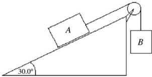
Two blocks are connected by a string that goes over an ideal pulley as shown in the figure. Block A has a mass of 3.00 kg and can slide over a rough plane inclined 30.0° to the horizontal. The coefficient of kinetic friction between block A and the plane is 0.40. Block B has a mass of 2.77 kg. What is the acceleration of the blocks?
