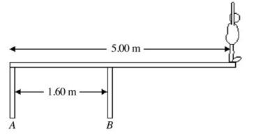
An 82.0 kg-diver stands at the edge of a light 5.00-m diving board, which is supported by two narrow pillars 1.60 m apart, as shown in the figure.
