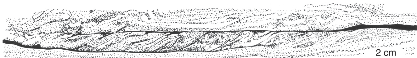
Figure 16.9 Imbrication zone formed in the overlap zone between two mica-rich layers (black) in mylonitic gneiss. The zone formed as displacement on the lower mica-rich layer was transferred to the upper one. From Rykkeliid & Fossen (1992).
