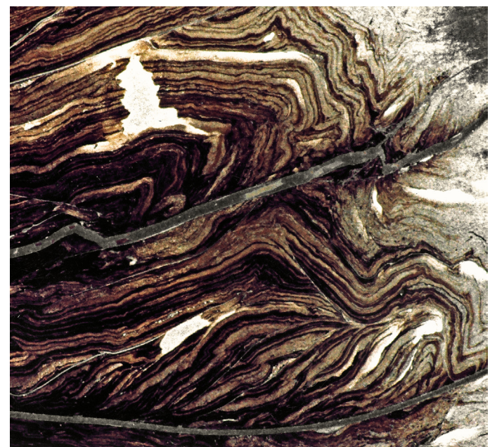
Figure 16.7 Micro-scale thrust structures and related folds (thin section). These structures, including roof thrusts, floor thrusts and horses, are similar to those found at much larger scale. Tertiary thrust zone in Carboniferous shales, Isfjorden, Svalbard. Picture is 2 cm wide. Photo: Steffen Bergh.
