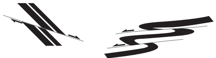
Figure 16.2 Contractional faults that at the same time are normal faults. They are contractional because they shorten or contract the layers that they affect.
