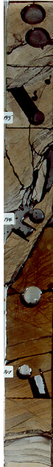
Figure 8.22 1 m long core section across a minor (6 m missing section) fault in the Gullfaks Field. Holes are from plugs sampled for permeability analysis.
