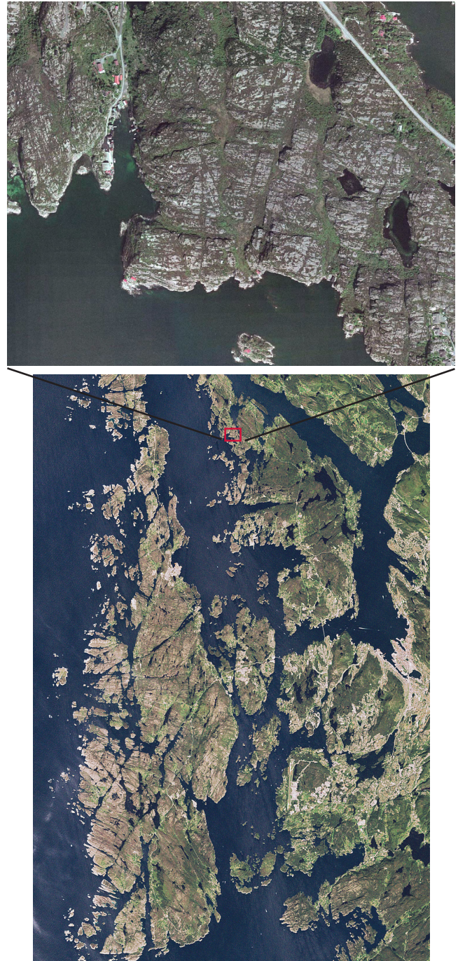
Figure 1.4 a) Landsat image over an area west of Bergen, Norway, and a more detailed aerial photo of a selected part of the satellite image. Satellite images are useful for regional analysis of fracture systems and foliations, while aerial photos are used for more detailed analyses.
